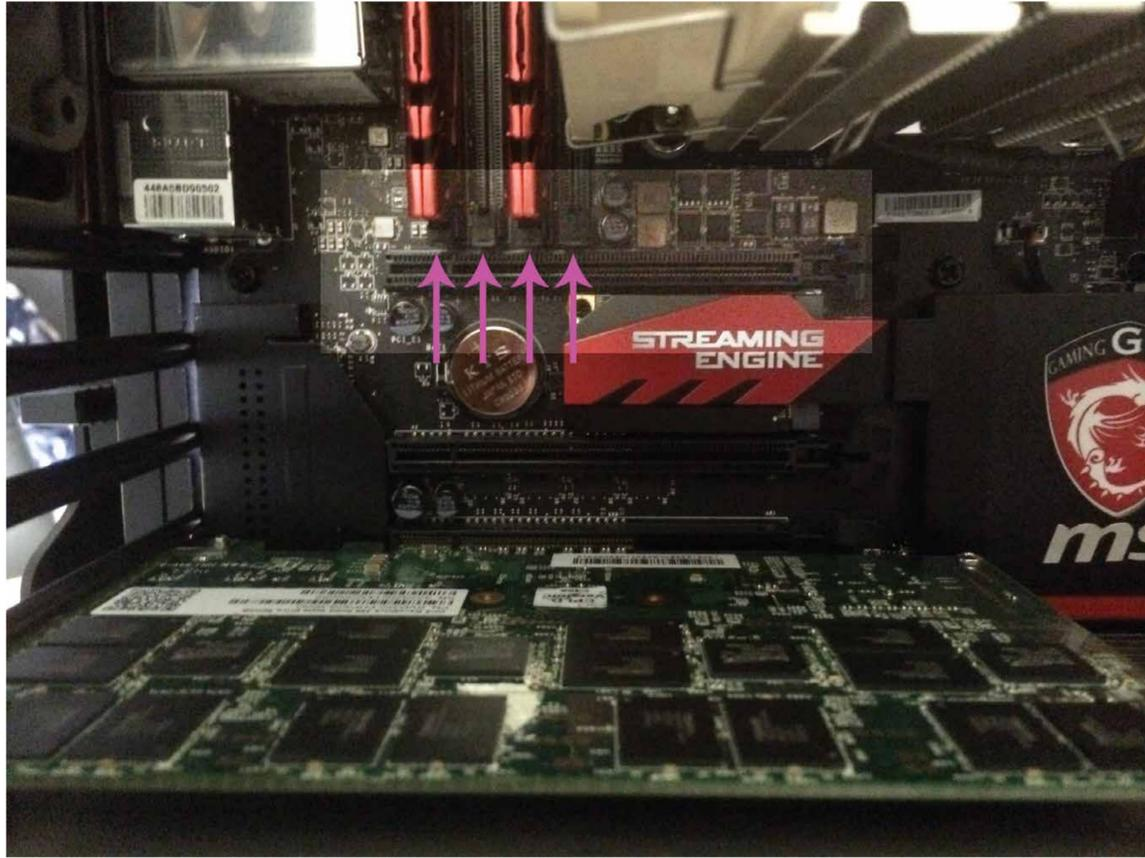
The Plastic support clips at the bottom of the ram module bays.
